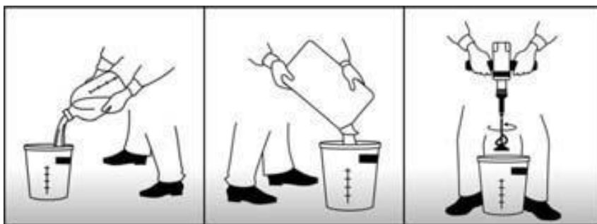
Figure 9 Mortar mix preparation
